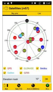
• To change the value of elevation mask shown at the bottom of the screen, just touch the current value and type in the desired value. Then touch **OK** to validate the new value.
