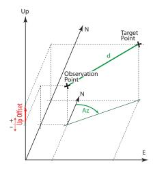
If unknown, the azimuth may be determined by Survey Mobile, directly in the field, **by specifying two points aligned with the target point** (see diagram below). In this case you have two observation points instead of just one. These points are named as follows:
